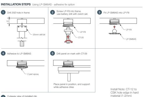
Cutaway view of installed clip (panel removed)
