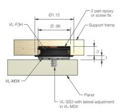
Through section showing surface mounted adhesive installation
