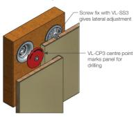
4 Section through recessed installation
