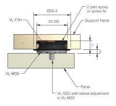
Through section showing surface mounted adhesive installation
